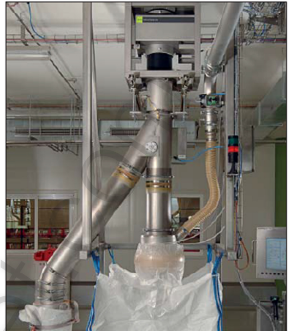
IFS compliant metal detection directly before the filling of spice products into bigbags
